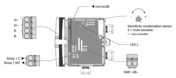
The relay is energized in the operating state (relays NO and C connected). Upon dew permeation or when the operating voltage is switched-off, the relay falls off.
